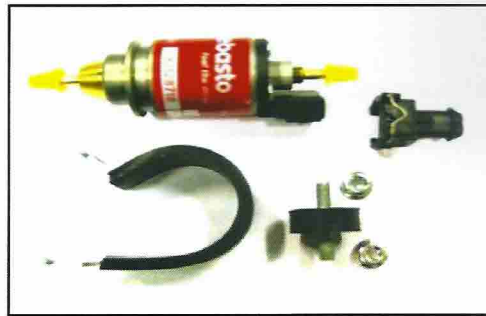
Fig 20 – Fuel pump, vibration dampener and mounting kit supplied in the kit.
